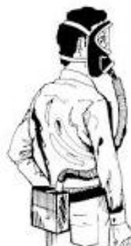
A self-contained breathing apparatus (SCBA) uses its own air tank and is used for entry and escape from atmospheres considered immediately dangerous to life and health or oxygen-deficient environments.
